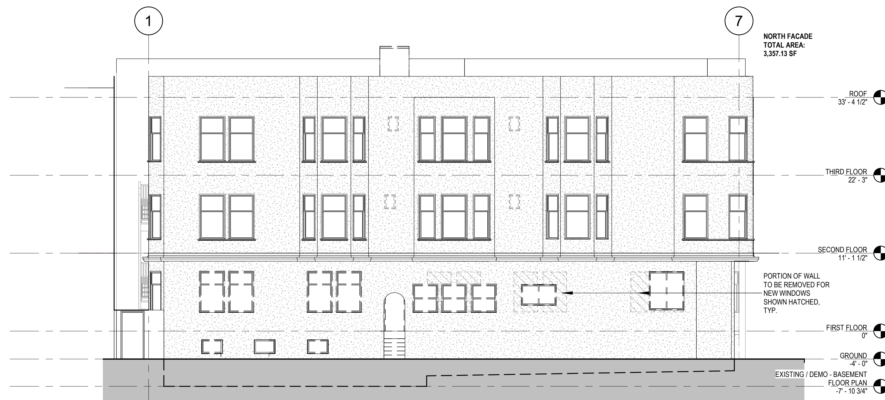
2 DEMO ELEVATION - NORTH (HERMANN STREET) 1/8" = 1'-0"
