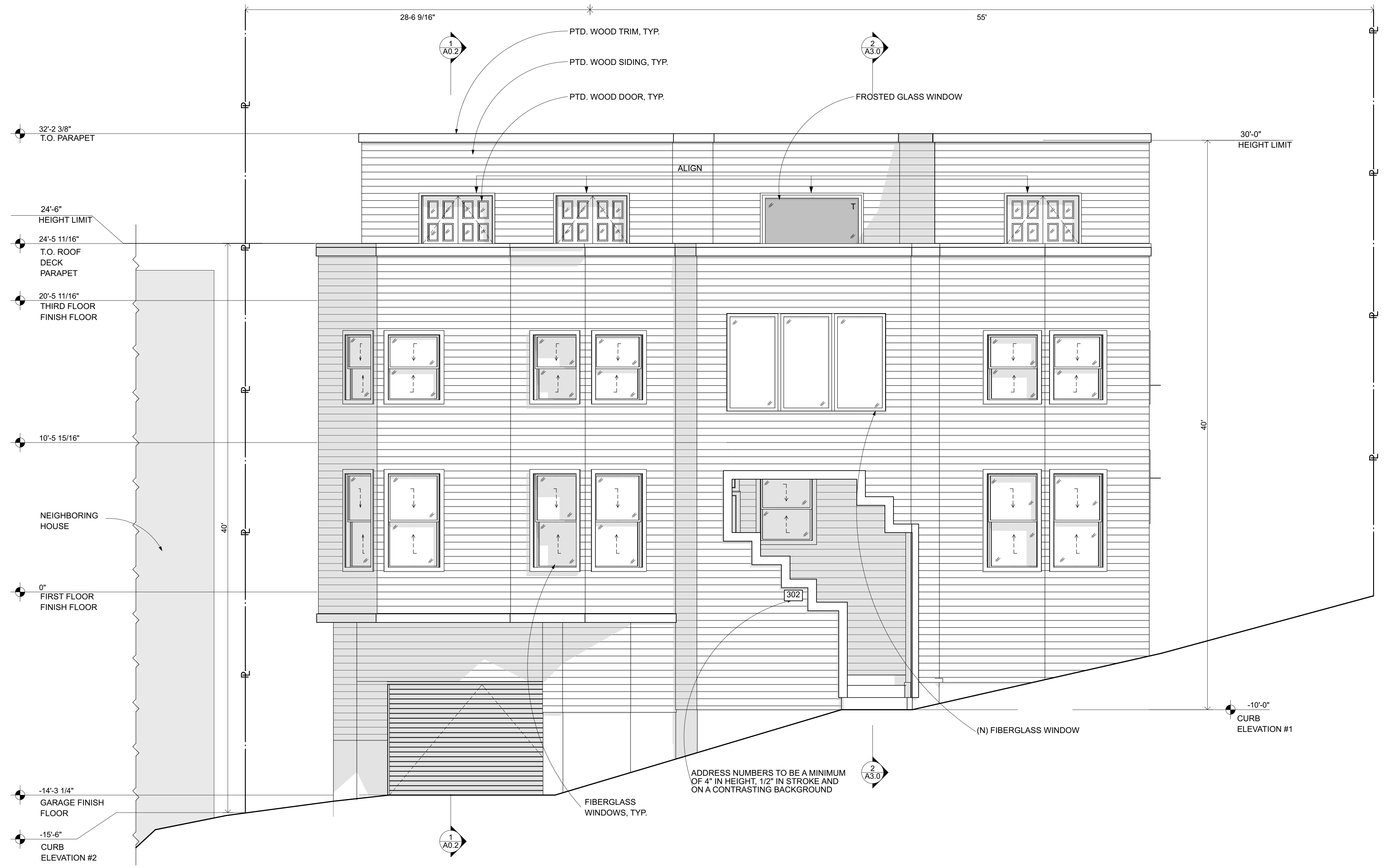
1 A2.1 ALTERED STREET SIDE ELEVATION SCALE: 1/4" = 1'-0"
