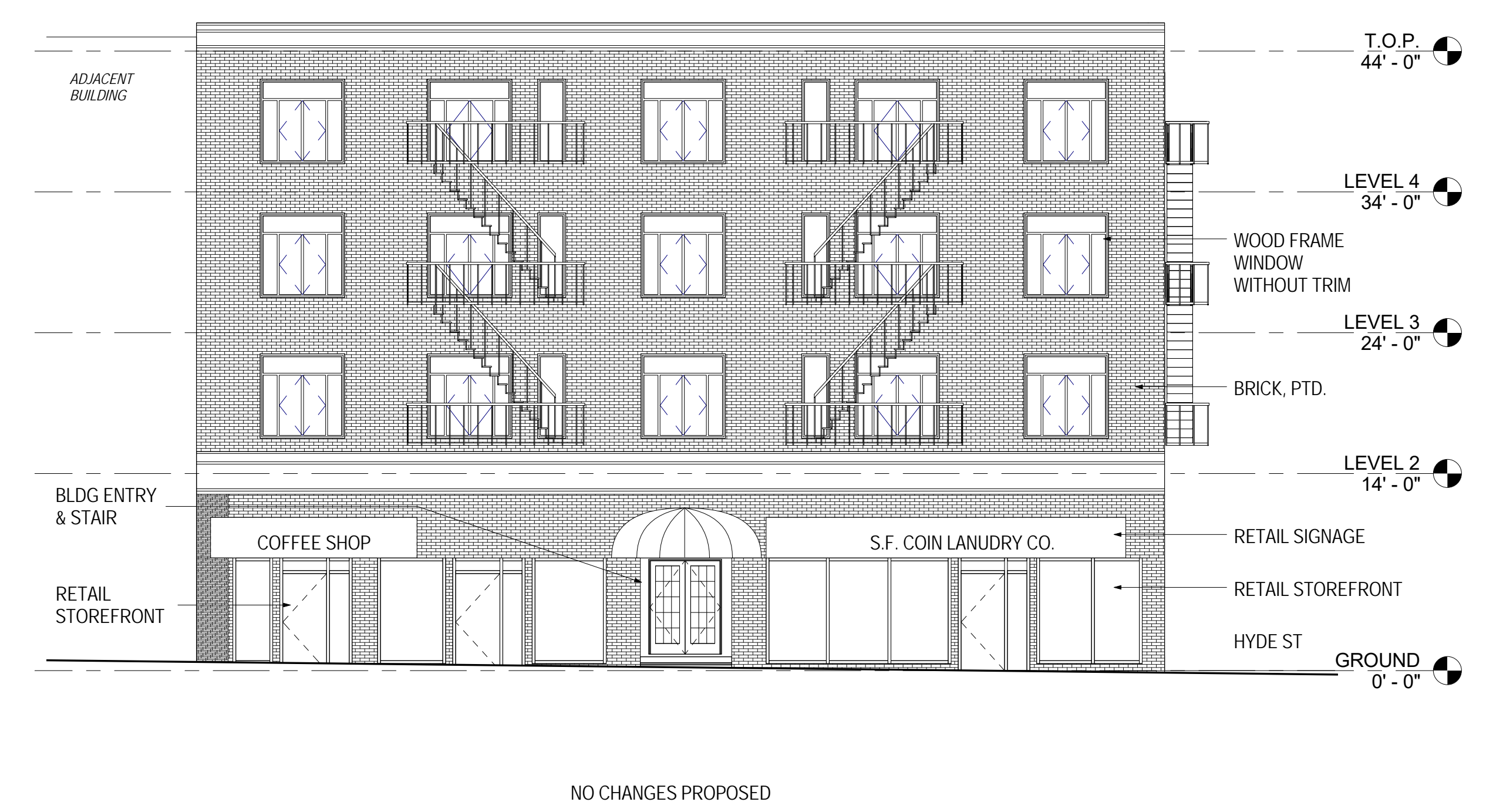
1/8" = 1'-0" FRONT ELEVATION - EXISTING (POST ST) 1
