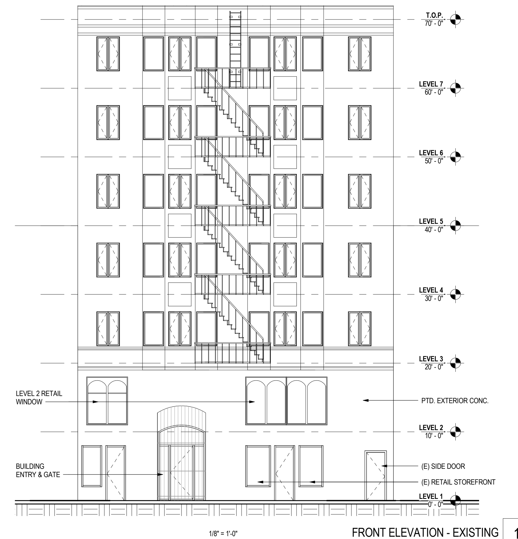
FRONT ELEVATION - EXISTING 1
