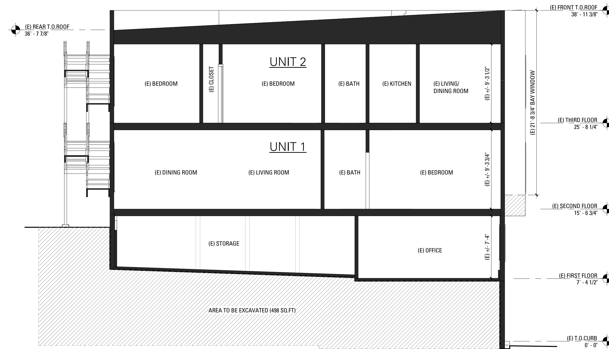
1 EXISTING BUILDING SECTION 3/16" = 1'-0"
