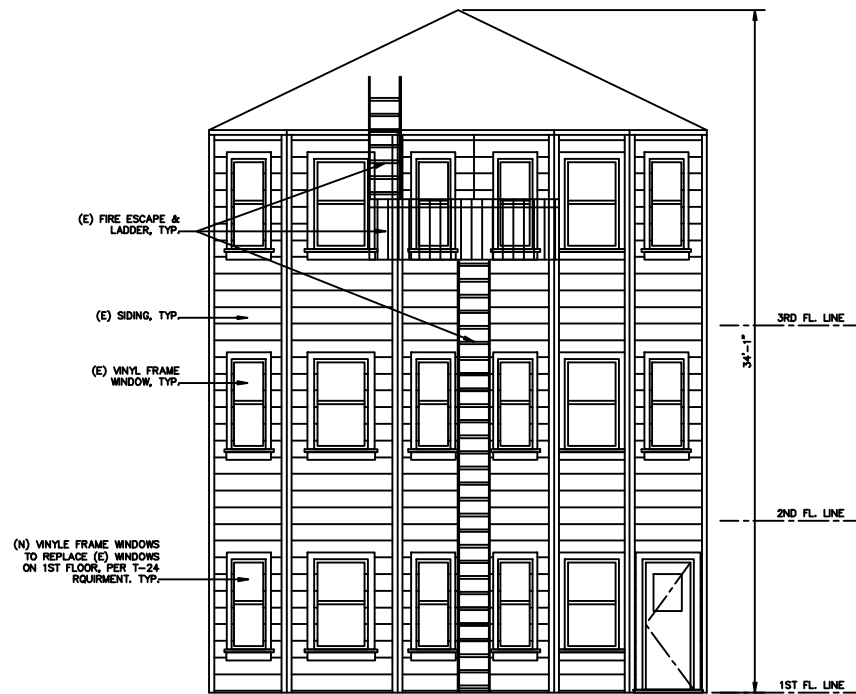
2 REMODEL REAR ELEVATION 1/4" = 1'-0"
