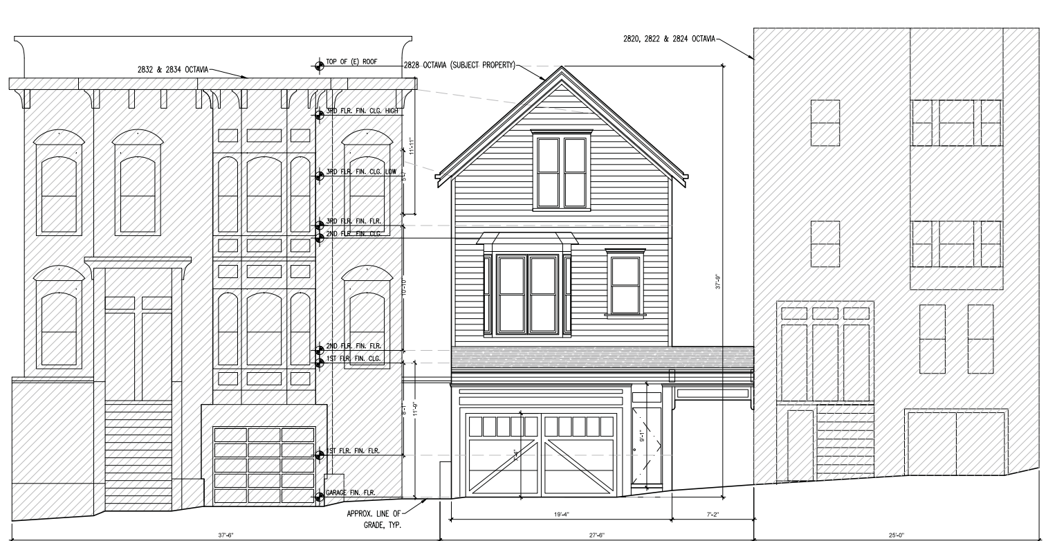
① WEST ELEVATION - EXISTING SCALE: 3/16" = 1'-0"
