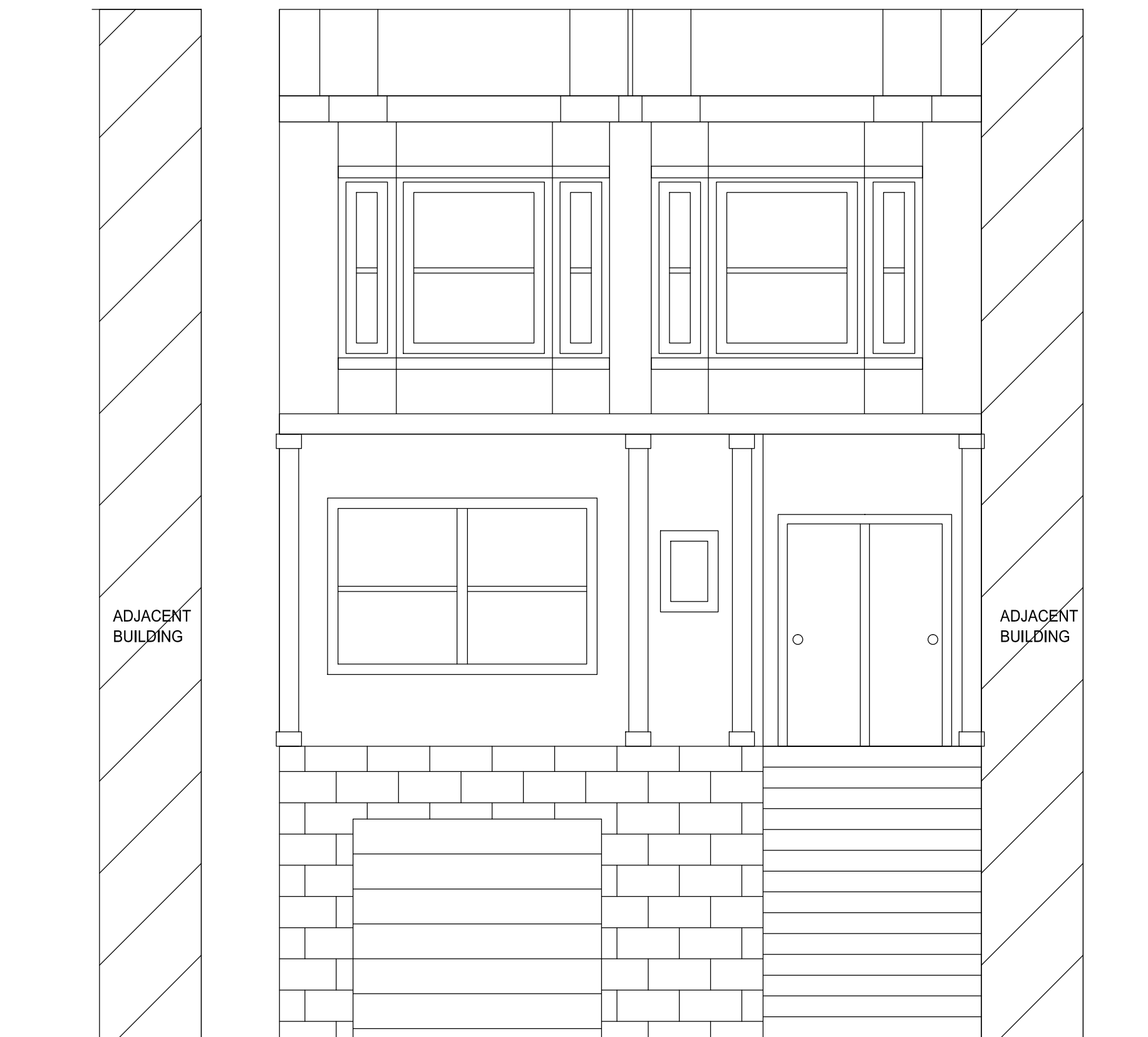
01 (E) FRONT BLDG. WEST ELEVATION A6 SCALE:1/4":1'-0"
