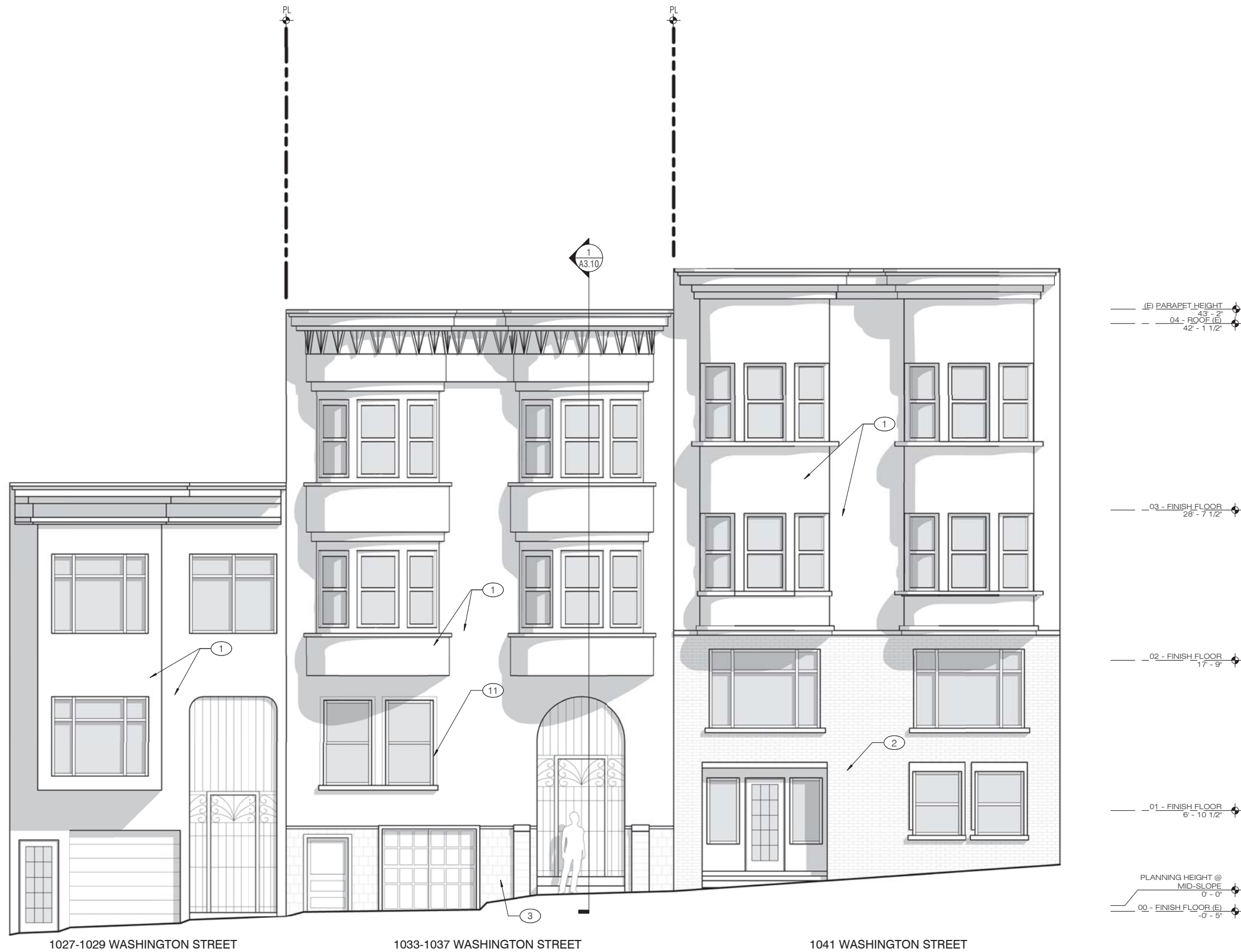
1 A3.00 EXISTING NORTH ELEVATION 1/4" = 1'-0"
