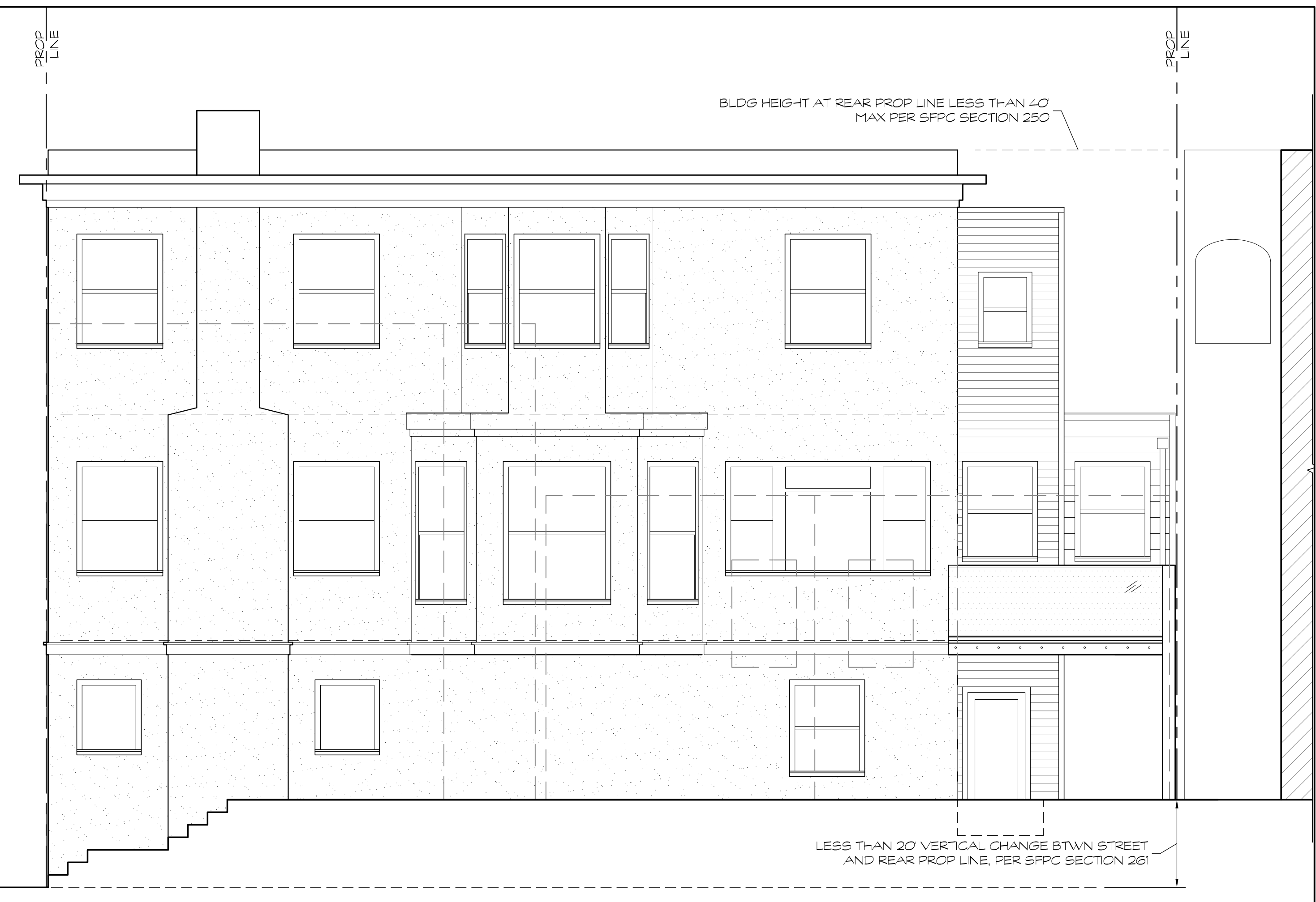
EXISTING EXTERIOR ELEVATION - SOUTH 1/4" = 1'-0" 3
